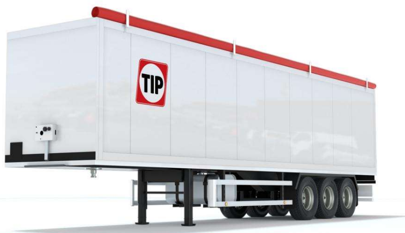
Figure 3-2 Example of "walking floor" trailer with canvas cover
